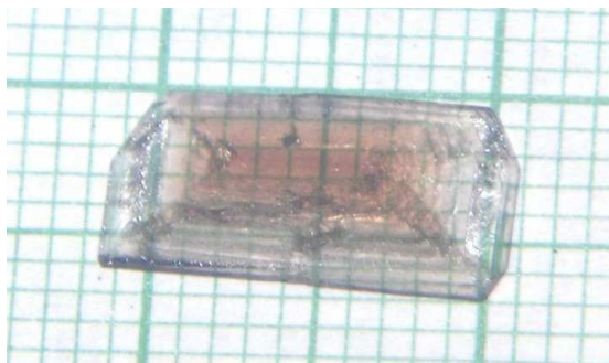
Fig.1 Photograph of as grown crystal of 4MAL
