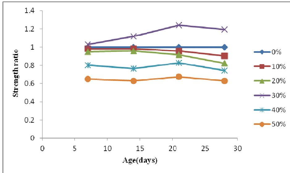
Figure 3. Relative compressive strength of concrete
