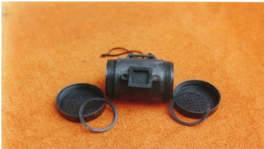
**Fig.-1 Photograph and Schematic diagram of radon- thoron twin chamber dosimeter cup**
