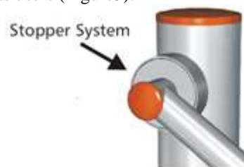
Figure5. Installation of stopper system on equipment
