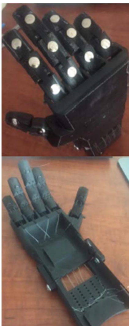
Figure 1: Assembled 3D printed prosthetic hand.
